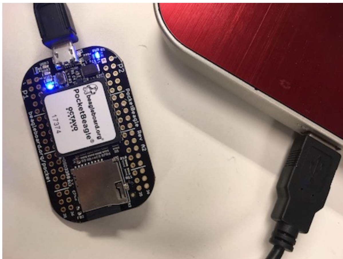
Fig. 3.12: Insert the USB connector into PC
