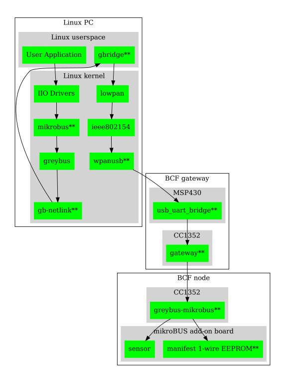
Fig. 3.1: BeagleConnect Software Architecture Diagram
