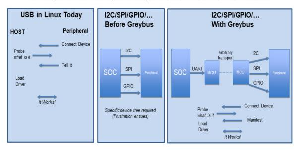
BeagleConnect<sup>™</sup> uses Greybus and mikroBUS add-on boards with ClickID and BeagleConnect<sup>™</sup> mikroBUS manifests to eliminate the need to add and manually configure devices added onto the Linux system.
